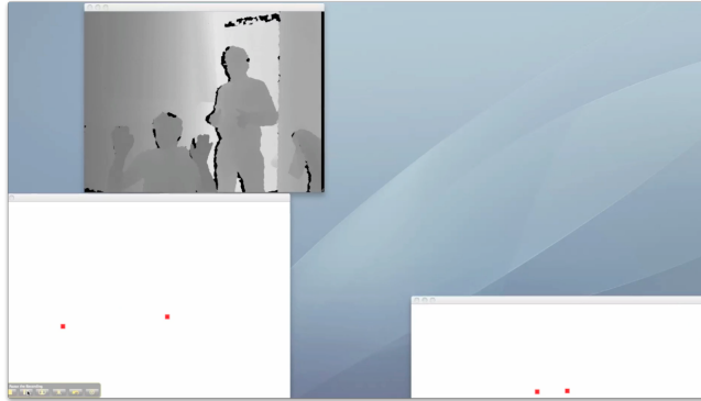
Figure 2: In this picture, users are tracked and each movement of both hands as well as that of the user's center of gravity is mapped to a dedicated window.
