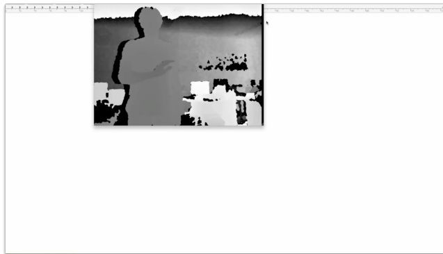
Figure 3: interaction with regular application, user movements are mapped to a mouse pointer, the location of the window can also be manipulated by the user's location.
