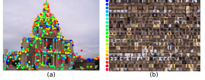
Fig. 2. Elementary blocks of Les Invalides . (a) SIFT keypoints are represented by circles; each color corresponds to a cluster. (b) Each row contains 25 sample patches from a given cluster.
