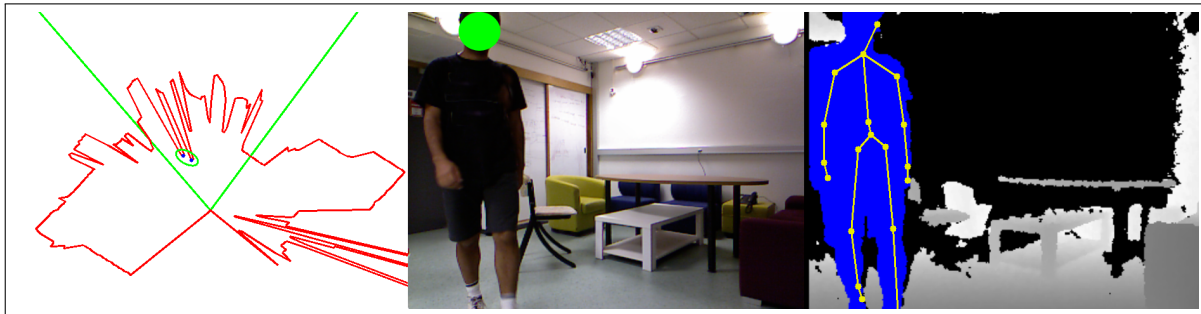
Figure 5: Perception from the robot point of view with a coming user toward a robot. Laser Telemetry (red lines), foot (blue spots) and pedestrian (green ellipse) information are depicted on left picture. In the middle, one can find RGB view from the Kinect with face detection (green circle). Right, the depth view with user (blue) and skeleton (yellow) tracking are drawn (note that with the first Kinect version, Kinect for Xbox , there is a little shift between the RGB and depth views). Acoustic and other body features are computed on these data (see section 4).
