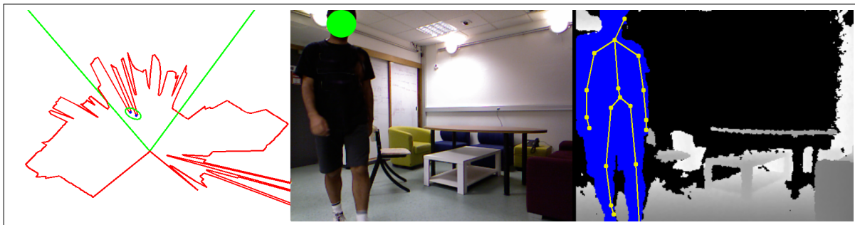
Figure 5: Perception from the robot point of view with a coming user toward a robot. Laser Telemeter (red lines), foot (blue spots) and pedestrian (green ellipse) information are depicted on left picture. In the middle, one can find RGB view from the Kinect with face detection (green circle). Right, the depth view with user (blue) and skeleton (yellow) tracking are drawn (note that with the first Kinect version, Kinect for Xbox , there is a little shift between the RGB and depth views). Acoustic and other body features are computed on these data (see section 4).
