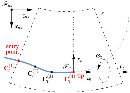
Fig. 1. Representation of the needle as a polynomial curve with 4 control points. Controlling the translational velocity  $v_z$  and the rotational velocity  $\omega_z$  allows the adjustment of the radius of curvature  $r$  of the trajectory.  $\mathcal{F}_n$  represents the frame attached to the needle tip, and  $\mathcal{F}_{us}$  the frame attached to the ultrasound volume.
