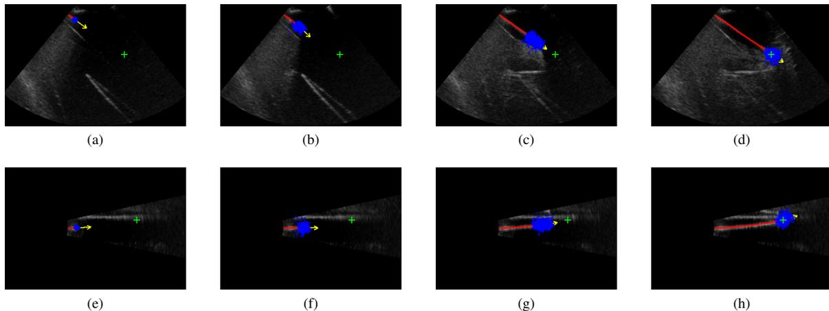
Fig. 3. Position of the needle in the ultrasound volume during automatic insertion, presented as a projection in the  $x$ - $z$  (a-d) and  $y$ - $z$  (e-h) plane. The needle detected by the tracker is represented as a red line, and the target as a green cross. The yellow arrow corresponds to the direction vector of the needle at the tip, and the blue points represent the position of the needle tip for all particles.
