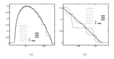
Figure 13: Variance for the cell-averaged solution of the inviscid Burgers equation at the final time t = 0.6. Two different zooms in the shock region are reported. The physical mesh is constituted by 601 equally spaced points.
