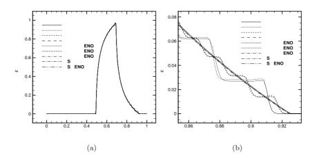
Figure 7: Expectancy for the cell averaged solution of the linear advection equation with discontinuous initial condition (63) at the final time t = 0.4. The whole physical domain is represented in (a), while in the figure (b) a zoom in the shock region is reported. The mesh is constituted by 601 equally spaced points.
