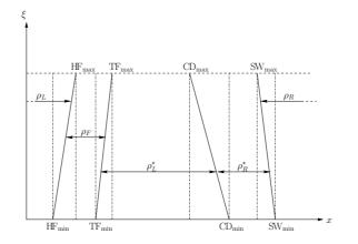
Figure 20: Schematic representation of the density of the uncertain shock tube problem in the combined physical/stochastic space. The regions where the solution should be subdivided are reported with the explicit identification of all the zones defining the variation of the solution as a function of the uncertain parameter  $\xi$ .
