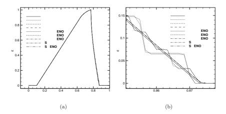
Figure 12: Expectancy for the cell-averaged solution of the inviscid Burgers equation at the final time t = 0.6. The whole physical domain is represented in (a), while in figure (b) a zoom in the shock region is reported. The physical mesh is constituted by 601 equally spaced points.
