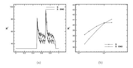
Figure 9: Evolution of the number of stochastic cells employed in each physical location for the aSI scheme with and without the ENO reconstruction (a) for the linear advection equation with discontinuous initial condition. The average number of stochastic cells employed by the aSI scheme as function of the physical space resolution is reported in (b).
