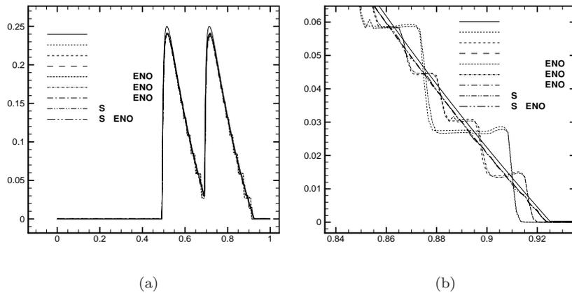
Figure 8: Variance for the cell averaged solution of the linear advection equation with discontinuous initial condition (63) at the final time  $t = 0.4$ . The whole physical domain is represented in (a), while in the figure (b) a zoom in the shock region is reported. The physical mesh is constituted by 601 equally spaced points.
