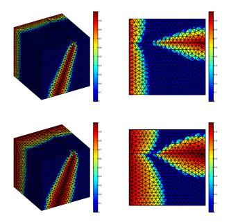
Figure 10: Inclined fracture: saturation of the injected wetting fluid at two different times. At left saturation on  $\partial \Omega$ . At right saturation on the bottom face of  $\Omega$ .
