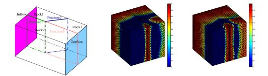
Figure 11: Left: Three intersecting fractures, no flow except through the magenta inflow region and the blue outflow region, higher permeability in fracture 2 than in fractures 1 and 3. Right: saturation at two different times.
