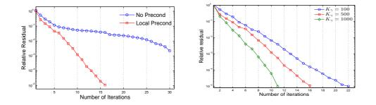
Figure 8: Efficiency of the CG preconditioner.
