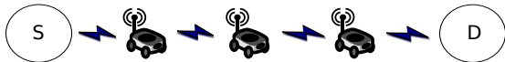
Fig. 4. Multiple routers scenario composed of three mobile routers, one source node, and one destination node.
