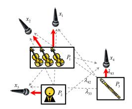
**Fig. 1.** Illustration of setup with three voices (violin section, flute, vocal soloist). Each voice is associated with at least one of the microphone channels. A solid line indicates a signal from a voice to its corresponding microphone, and a dashed line indicates an interference signal from other voices into a microphone.
