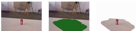
Fig. 18. Regions around the measured depth are assumed to be foreground objects (Eq. 33). Green points are projection of samples with p_s^f > 0.8 .
