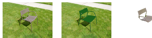
Fig. 14. Results on the Chair [30] dataset (using 4 views). Green points indicate projection of samples with high foreground probability. Last column is the final segmentation, with thin legs being lost while they were correctly labeled at the sparse samples level.
