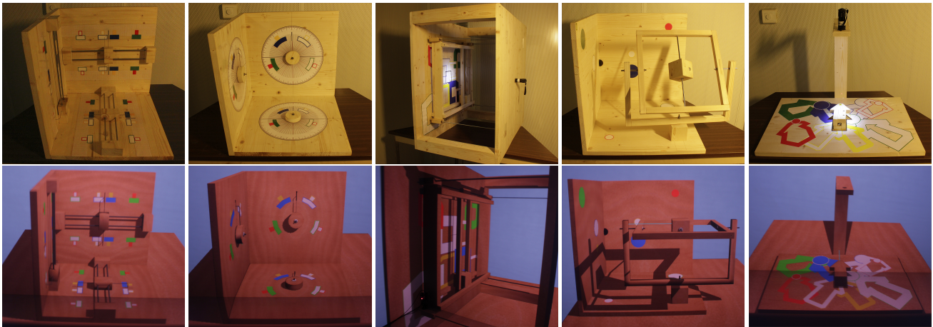
Figure 2: Devices used to decompose motion. From left to right: 1 DoF translations, 1DoF rotations, 3DoF translations, 3DoF rotations, free (6DoF) movements. The top line shows the physical devices, and the bottom line shows their virtual implementation.
