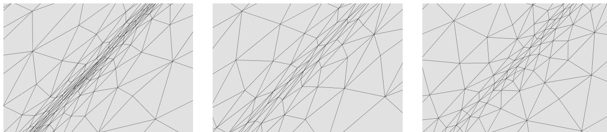
Figure 1. Example of mesh coarsening. Left: initial mesh. Middle: Isotropic coarsening. Right: Anisotropic coarsening.
