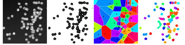
**Fig. 2.** Example of candidate shape generation with the four steps of RS-SKIZ method. From left to right: crop –  $340 \times 340$  px – of the initial synthetic image –  $950 \times 950$  px –, skeleton on the thresholded image, random seeds with associated SKIZ and obtained candidates.
