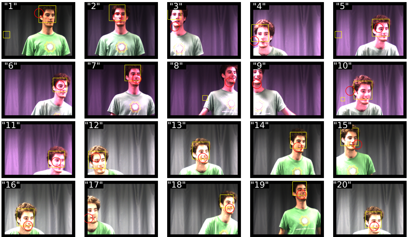
Fig. 4. The moving-speaker scenario. The person is static while he pronounces a number (written in white) and he moves between two numbers. The red circles show the position found with our method. The yellow squares correspond to faces detected with [21]. The full video is available at https://team.inria.fr/perception/research/binaural-ssl/ .
