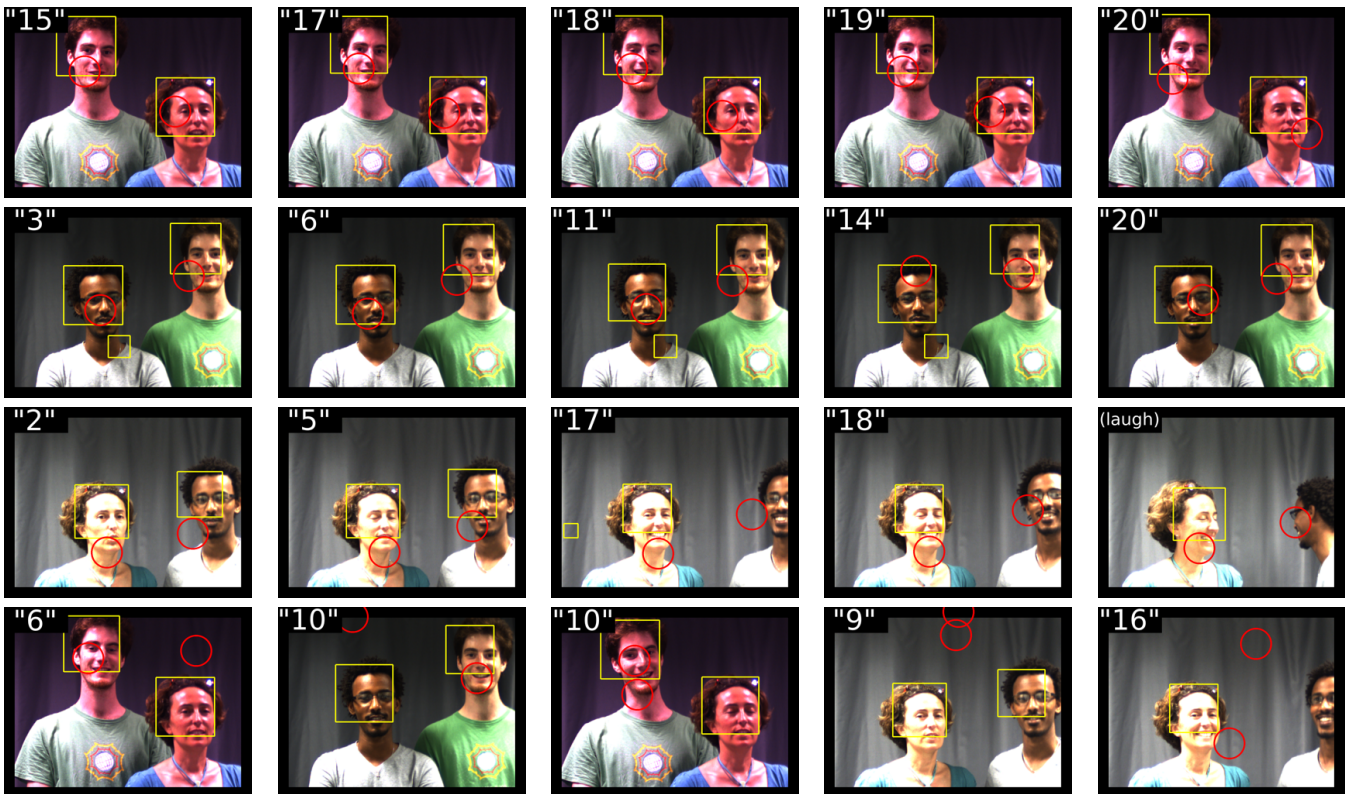
Fig. 7. Two subjects count from 1 to 20 (white numbers) in different languages, with a normal voice loudness, from a fixed position. The red circles show the position found with our method. The yellow squares show the results of the Viola-Jones face detector[21]. The first 3 rows show examples of successful localization results, the last row shows examples of typical localization errors. Full videos available at https://team.inria.fr/perception/research/binaural-ssl/ .
