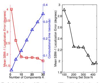
Fig. 3. Left: Influence of K on the mean GTEA and localization time of a 1 second speech source using the proposed supervised binaural mapping method (M=1,N=432). Right: Influence of N on the mean GTEA of a 1 second speech source (K=32).
