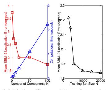
Fig. 6. Left: Influence of K on the mean GTEA and localization time of a 1 second S+S mixture using the proposed supervised binaural mapping method (M=2,N=20,000). Right: Influence of N on the mean GTEA of a 1 second S+S mixture (K=100).
