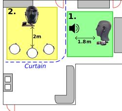
Fig. 2. Left: A typical recording session. The two microphones plugged into the ears of the dummy head are the only ones used in this paper, although the head is equipped with four microphones. Right: Top view of the recording room. The robustness of the method with respect to room changes is validated by using different locations for training with white noise emitted by a loudspeaker (green zone #1) and for testing with human speakers (yellow zone #2).
