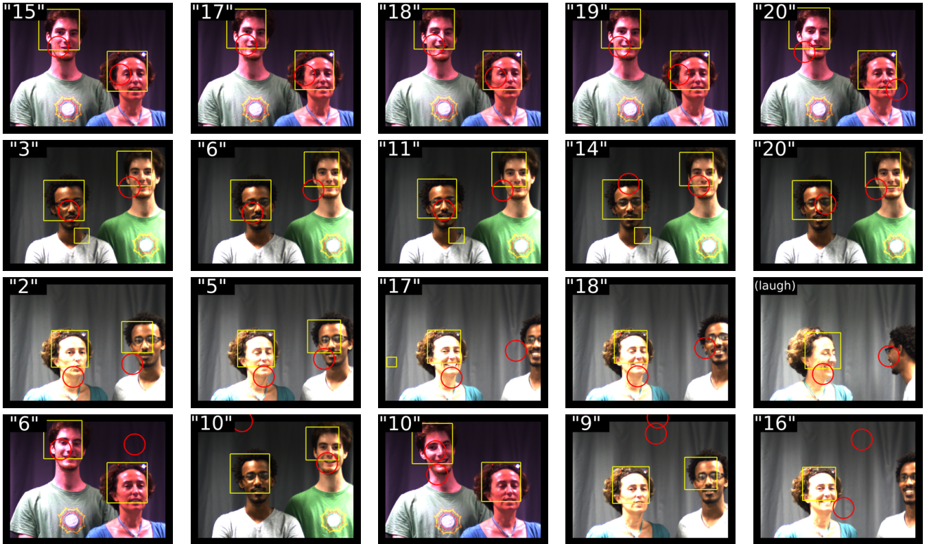
Fig. 7. Two subjects count from 1 to 20 (white numbers) in different languages, with a normal voice loudness, from a fixed position. The red circles show the position found with our method. The yellow squares show the results of the Viola-Jones face detector[21]. The first 3 rows show examples of successful localization results, the last row shows examples of typical localization errors. The full videos are available in supplementary materials.
