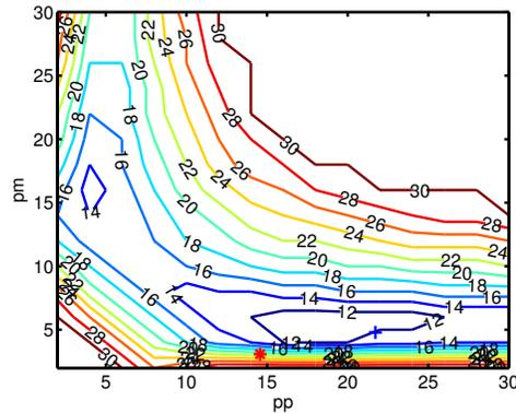
**Fig. 3.** Level curves for the number of iterations needed to reach convergence for various values of the parameters  $p^-$  and  $p^+$ . The lower left star marks the parameters derived from Theorem 5, whereas the upper right cross shows the "optimal" parameters, as found by numerically minimizing the continuous convergence rate.
