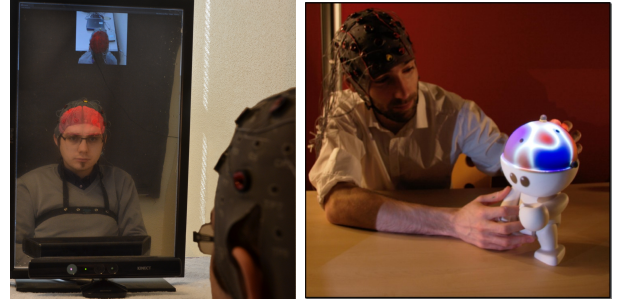
Fig. 4. Left: the Mind Mirror, Right: Teegi, two new real-time visualization tools of the user's own brain activity, based on augmented reality.
