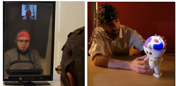
Fig. 4. Left: the Mind Mirror, Right: Teegi, two new real-time visualization tools of the user's own brain activity, based on augmented reality.
