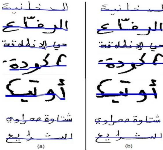
Fig. 3. (a) Extracted baseline, (b) baseline by horizontal projection
