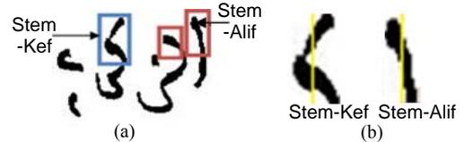
Fig. 6. (a) Ascender extraction (b) Ascender classification based on number of white to black or black to white pixel transitions.
