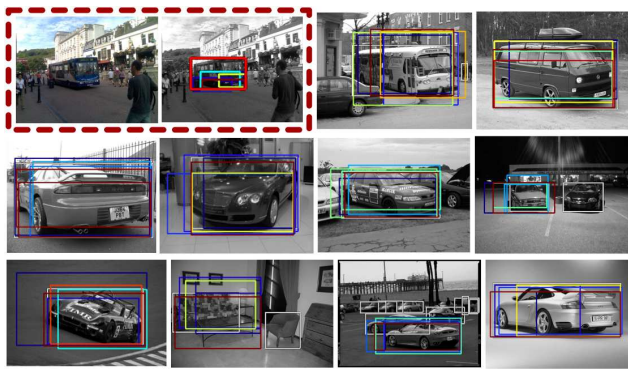
Figure 9. Localization in an example and its neighbor images on mixed-class PASCAL07-all. A bus is successfully localized in the image (red dashed box) from its neighbors (10 images) containing even other classes (car, sofa). Boxes in the neighbors show potential object regions at the final iteration. (Best viewed in color.)
