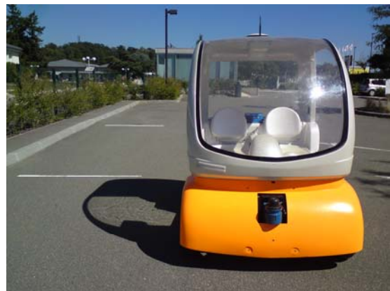
Figure 1. The automated CyCab vehicle developed at INRIA equipped with DGPS, odometers and laser range finder.
