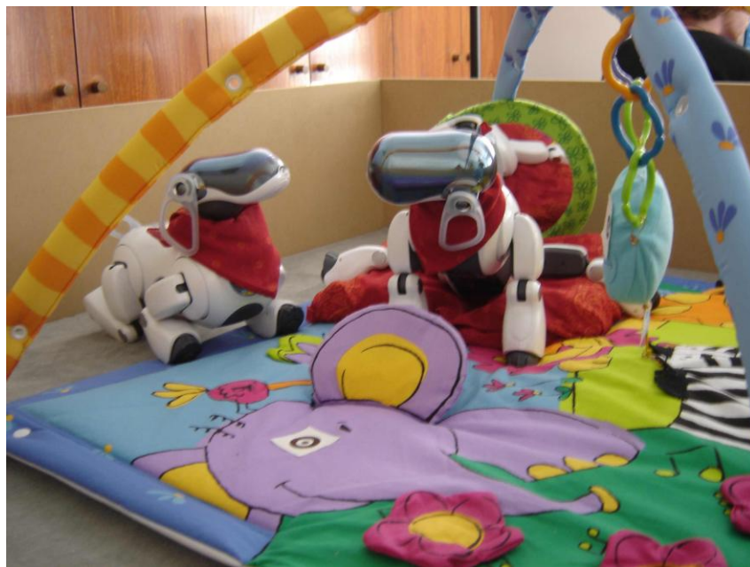
Figure 4 Curiosity-driven learning in the Playground Experiment. The Playground Experiment (Oudeyer et al., 2007 ; Oudeyer and Smith, 2014). The robot in the center explores and learns to predict the effects of its actions, driven by a form of artificial curiosity. The behaviors and know-how it acquires spontaneously evolve and self-organize into developmental stages of increasing complexity, without an initial program specifying these stages. For example, the robot learns at its own initiative how to grasp an object in front of him, or how to produce vocalizations which provoke reactions in the other robot.
