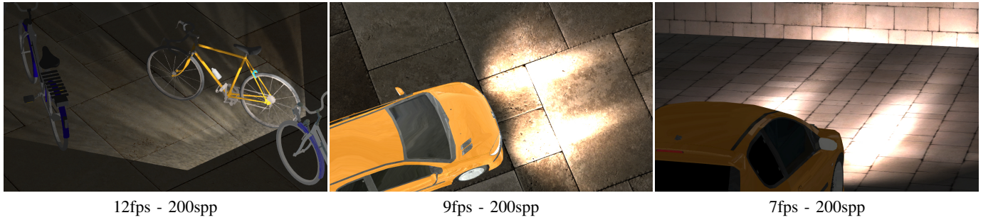
Fig. 2. Our new light importance sampling technique estimates, at interactive frame rate, direct lighting with only 200 samples per pixel (spp) that are distributed among the different images of the light field luminaire. (Left) The bike headlight light field contains 9 \times 7 images ( 300 \times 300 pixels). The visibility is computed with 80 shadow maps ( 256 \times 256 pixels). (Center and Right) The car headlights are represented by the same light field composed of 11 \times 9 images ( 256 \times 256 pixels).
