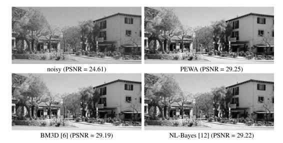
Figure 2: Comparison of algorithms. *Valldemossa* image corrupted with white Gaussian noise ( $\sigma = 15$ ). The PSNR values of the three images denoised with DCT-based transform [26] and combined with PEWA are 27.78, 27.04 and 26.26.
