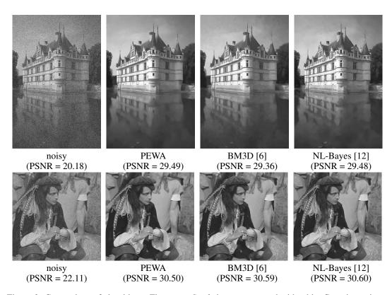
Figure 3: Comparison of algorithms. First row: *Castle* image corrupted with white Gaussian noise ( $\sigma=25$ ). The PSNR values of the three images denoised with DCT-based transform [26] and combined with PEWA are 25.77, 24.26 and 22.85. Second row: *Man* image corrupted with white Gaussian noise ( $\sigma=20$ ). The PSNR values of the three images denoised with DCT-based transform [26] and combined with PEWA are 27.42, 26.00 and 24.67.
