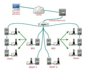
Fig. 7. An Interference Alignment scenario based on cognitive MIMO-OFDM transceivers.
