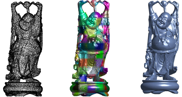
Fig. 1. IBS patches are reconstructed in small cells and blended together: (left) 3D point cloud of Buddha ; (middle) the overlapping IBS patches; (right) the blended IBS surface.
