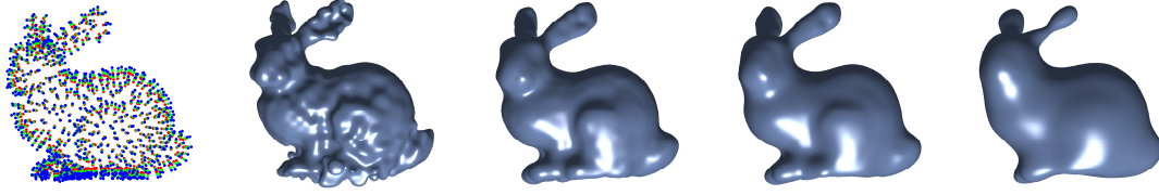
Fig. 4. The effect of regularization parameter in 3L-IBS method; (left) the offset of Bunny ( \delta = 1\% ); the rest from left-to-right: different settings for the regularization parameter \mu = 1, 10^2, 10^3, 10^4 respectively.
