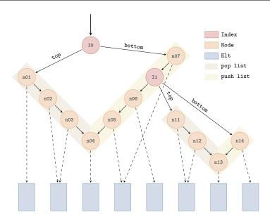
Figure 6: Example of a possible queue internal structure. Here, the main queue is accessible through the index 10. The index 11 is pointing to a queue concatenated during a previous merge operation. This queue will be unfolded during the next normalization. Because of the Irmin store behavior, two nodes containing the same element share its physical representation.
