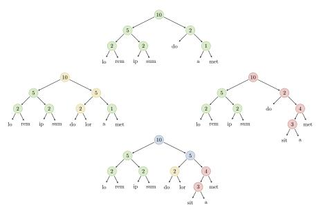
Figure 11: In this example, the old green rope have been modified in two different manners – yellow and red –, resulting in two ropes having to be merged. In this case, the merge algorithm is able to select the two relevant subtrees in both of the ropes, and returns the final rope without having to call the user-provided merge function.
