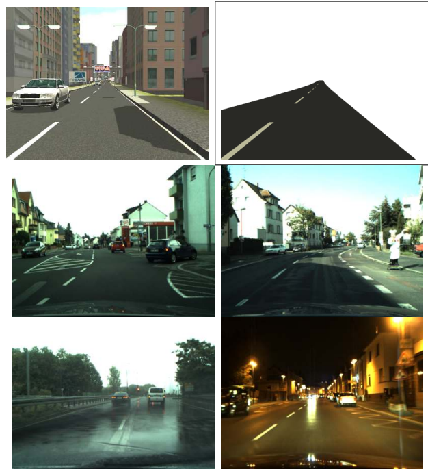
Fig. 2. Databases used for training and testing. Top row: simulated traffic image and corresponding road mask obtained from the simulation tool. Middle row, bottom row: images from substreams I,II,III,IV of the HRI RoadTraffic benchmark, corresponding to overcast/dry, low sun/dry, rain, and night conditions. Please note the realistic rendering of shadows on the road by the simulator as compared to similar shadows in stream II (middle row, right image).
