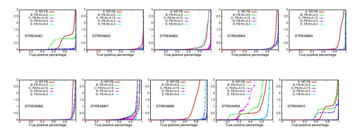
Fig. 4. Effect of dynamic attention priors on each of the 10 test streams. In each plot, there is either no feedback ( $\bf A$ ) or feedback where the tracker is fed only with detections that exceed confidence thresholds of 0 ( $\bf B$ ), 0.15 ( $\bf C$ ), 0.3 ( $\bf D$ ) and 0.4 ( $\bf E$ ). A strong overall improvement of detection rates is clearly observable.
