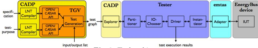
Fig. 2. Tool architecture
