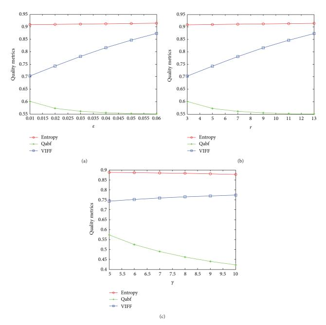
FIGURE 7: Analysis of different free parameters used in the algorithm. Maximum quality score and entropy are only observed when  $\varepsilon = 0.01$ ,  $\gamma = 5$ , and r = 2 (which are set as default parameters). It is observed that VIFF increases as  $\varepsilon$ ,  $\gamma$ , and r increases but the larger values are responsible for overenhancement. (a) Effectiveness of  $\varepsilon$  on metrics, (b) effectiveness of r on metrics, (c) effectiveness of  $\gamma$  on metrics.
