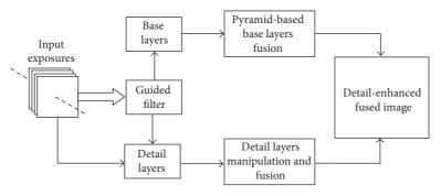
FIGURE 2: Proposed detail-enhanced exposure fusion framework.
