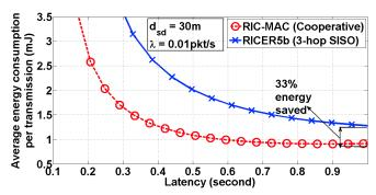
Fig. 6. Comparison of energy consumption between multi-hop and cooperative relay using real MAC protocols (energy models based on PowWow platform) in low traffic load networks
