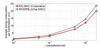
Fig. 9. Energy consumption of cooperative RIC-MAC and 3-hop RICER5b at  $T^{opt}$  versus  $\lambda$
