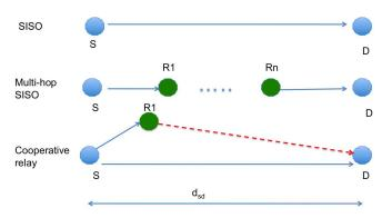
Fig. 1. SISO, multi-hop SISO and cooperative relay models
