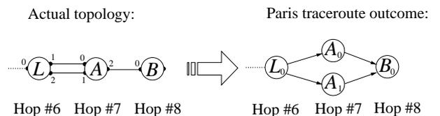
Figure 7: Load balancing over parallel links
