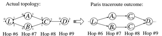
**Figure 5: The IP-level multi-path inferred by Paris traceroute may not correspond to the router-level multi-path in the real topology.**
