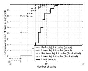
Figure 1: Path diversity in the Sprintlink topology.
