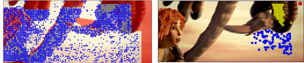
Figure 6. Left: Match positions returned by [34] are shown in blue. Red denotes occluded areas. Right: Yellow (resp. blue) squares correspond to the 100 nearest matches with a Euclidean (resp. edge-aware geodesic) distance for the occluded pixel shown in red. All neighbor matches with a Euclidean distance holds to a different object while the geodesic distance allows to capture matches from the same region, even in the case of large occluded areas.
