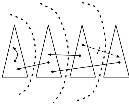
Figure 3: The principle of Kosaraju's algorithm.  $f_1$  is a DFS forest for the graph  $E$ .  $f_2$  is a DFS forest for the reverse graph  $\bar{E}$ . The vertex  $r$  is the root of the last tree in  $f_1$  and the root of the first tree in  $f_2$ . The component  $scc(r)$  forms a prefix of the last tree in  $f_1$  and is exactly the first tree in  $f_2$ .
