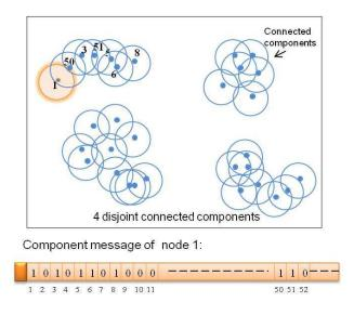
Figure 15: Bitmap of node 1 in its Component message.
