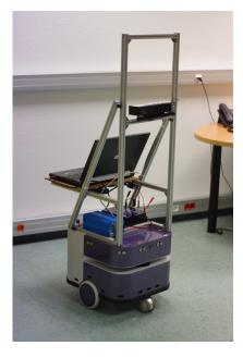
Fig. 1. Robotic platform used for recording: a Robulab10 mobile robot from the Robosoft compagny. It is equipped with a laser ranger finder, a Kinect 2.0 and a laptop computer.
