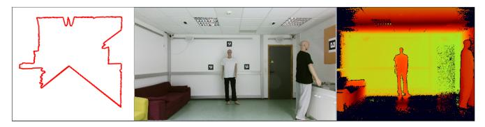
Fig. 8. Robot sensor view. At left, the laser range finder view. In the middle, the RGB stream. Last, the infrared view. The depth view (not on this figure) is aligned with the infrared one.
