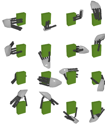
Figure 6: The set of all the grasping directions computed for a box-shaped object. Other poses are obtained by adding small offsets in the main axis directions, for a total of 144 grasps. The fingers are represented closed on the object as they are when the feasibility of a grasp is evaluated.
