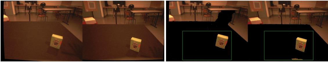
(a) The original images after distortion removal.
