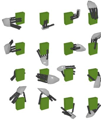
Figure 6: The set of all the grasping directions computed for a box-shaped object. Other poses are obtained by adding small offsets in the main axis directions, for a total of 144 grasps. The fingers are represented closed on the object as they are when the feasibility of a grasp is evaluated.
