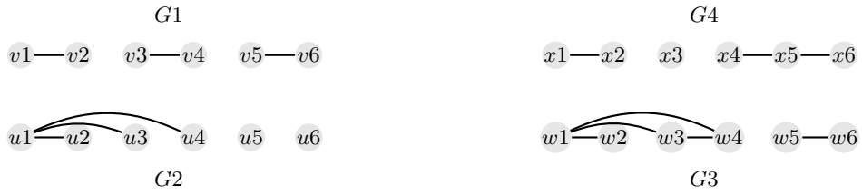
Fig. 2. Consider graphs G_1, \dots, G_4 . It is easily seen that \text{CMO}(G_1, G_2) = 1 , \text{CMO}(G_2, G_3) = 3 and \text{CMO}(G_1, G_3) = 3 . We then obtain: D_{\text{sum}}(G_1, G_2) = 1 - \frac{2}{|E_1| + |E_2|} = 1 - \frac{2}{6} = \frac{2}{3} , D_{\text{sum}}(G_2, G_3) = 1 - \frac{6}{|E_2| + |E_3|} = 1 - \frac{6}{8} = \frac{1}{4} , D_{\text{sum}}(G_1, G_3) = 1 - \frac{6}{|E_1| + |E_3|} = 1 - \frac{6}{8} = \frac{1}{4} . Hence D_{\text{sum}}(G_1, G_3) + D_{\text{sum}}(G_3, G_2) = \frac{1}{2} < \frac{2}{3} = D_{\text{sum}}(G_1, G_2) . Furthermore, \text{CMO}(G_2, G_4) = 1 and \text{CMO}(G_3, G_4) = 2 . We then obtain: D_{\min}(G_2, G_4) = 1 - \frac{\text{CMO}(G_2, G_4)}{\min\{|E_2|, |E_4|\}} = 1 - \frac{1}{3} = \frac{2}{3} and D_{\min}(G_3, G_4) = 1 - \frac{2}{3} = \frac{1}{3} , as well as D_{\min}(G_2, G_3) = 1 - \frac{3}{3} = 0 . Hence, D_{\min}(G_2, G_3) + D_{\min}(G_3, G_4) = 0 + \frac{1}{3} < \frac{2}{3} = D_{\min}(G_2, G_4) .
