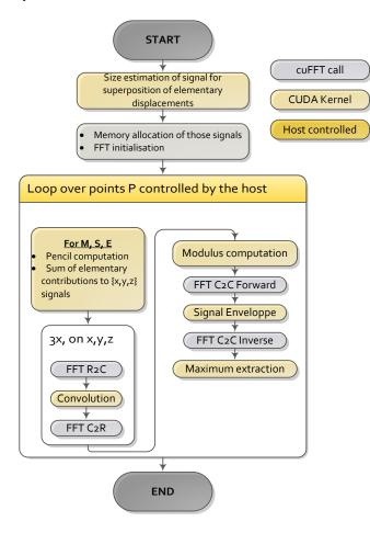
Figure 6 - Algorithm of the GPU implementation
