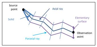
Figure 2 - Ray tube visualization
