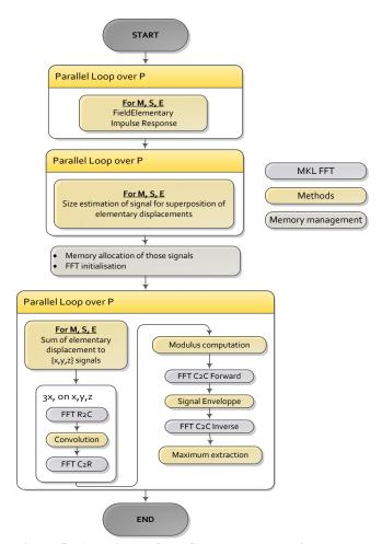
Figure 5 - Algorithm of the GPP Implementation
