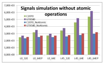
Figure 16 – GPU normalized time with and without atomic operations (C2070 and GTX580 only)
