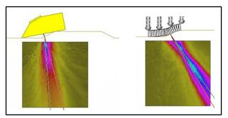
Figure 1 - Field simulation inside a weld with two different probes.
