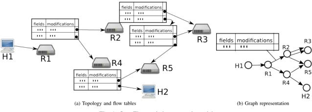
Fig. 1: OpenFlow switches network model
