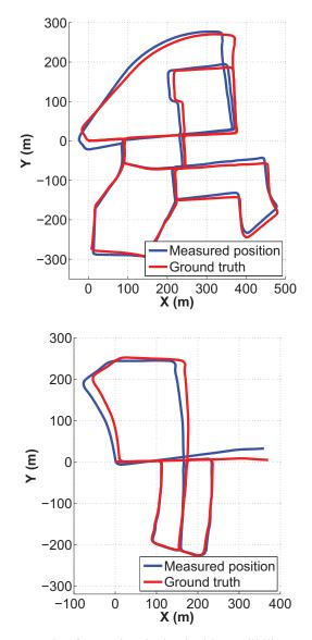
Fig. 6: Example of a results obtained with Credibilist SLAM on sequences from the KITTI database
