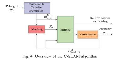
The obtained best match corresponds to the vehicle displacement so that both its trajectory and the surrounding map are estimated in the same process. Since the displacement alone leads to a relative localization only, the considered reference in this article is the vehicle reference  $R_0$  at the beginning of the experiment. It means that at any time t, the position of the vehicle (x, y) and its heading  $\theta$  are given relatively to the position and the heading at time t = 0.
