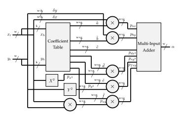
Fig. 8. Architecture based on a second order bivariate polynomial
