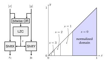
Fig. 4. Scaling range reduction
