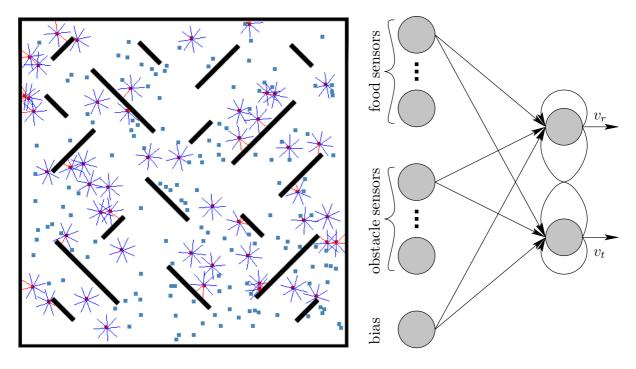
Figure 1: Left: the simulation environment containing agents (red dots with thin hairlines representing sensors), obstacles (dark lines) and food items (blue dots). Right: the architecture of the neuro-controller.
