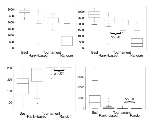
Figure 6: Box and whisker plots (30 independent runs) of the comparison measures for the four selection methods on the foraging task. From top to bottom and left to right:  $f_c$ ,  $f_b$ ,  $g_f$  and  $f_a$ . The label p > 0.01 indicates no statistical difference for the corresponding two selection methods.
