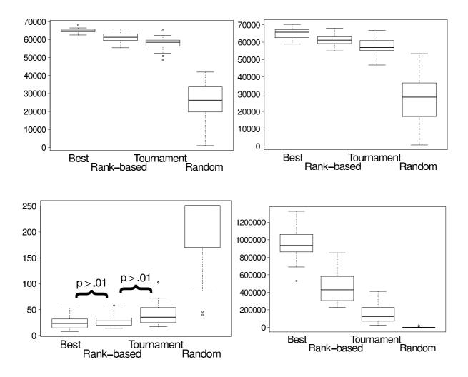
Figure 5: Box and whisker plots (30 independent runs) of the comparison measures for the four selection methods on the navigation task. From top to bottom and left to right:  $f_c$ ,  $f_b$ ,  $g_f$  and  $f_a$ . The label p > 0.01 indicates no statistical difference for the corresponding two selection methods.
