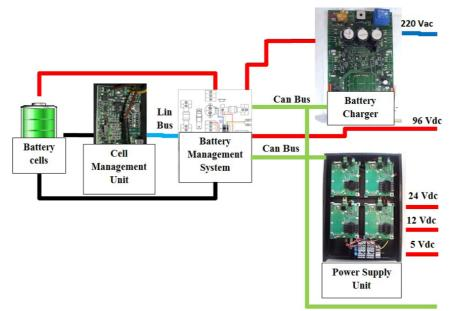
Figure 5 Sketch of the general architecture of the power supply (see online version for colours)
