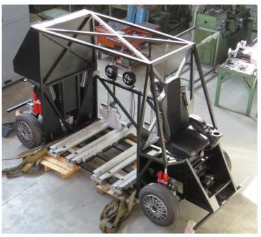
Figure 2 Prototype at shop testing (cover removed to show the inside) (see online version for colours)
