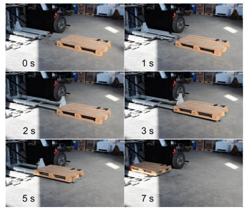
**Figure 3** FURBOT unloading cycle (from top to bottom, from left to right): intermediate positions of the fork loading an empty pallet (see online version for colours)
