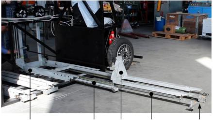
base intermediate slider fork fork slider wheels
